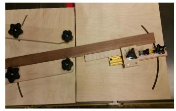
After setting the sled for the number of segments use a straight edge to set the stop block to the same angle as the lower fence and lock in position.
