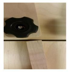
Adjust the stop block so the edge is over the kerf and lock in position. Then cut off the edge to create the same angle as the segments. This will need to be done each time the sled is set to a different number of segments. The stop block is sacrificial and can easily be replaced. Use the front miter track runner adjusting screw to hold the table in position at the front edge of the table saw table. Do not over tighten this may strip the threads.
